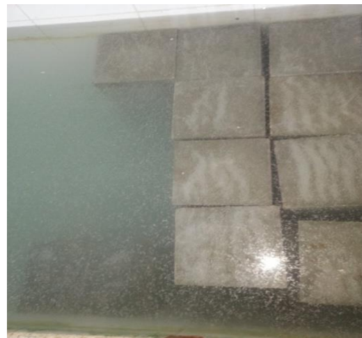
Figure 3.11 : Cubes at curing basin
