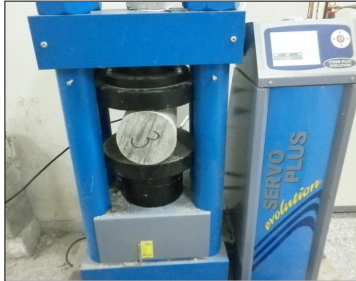
Figure 3.13: Split cylinder test setup for cylinder 150 x 300mm
