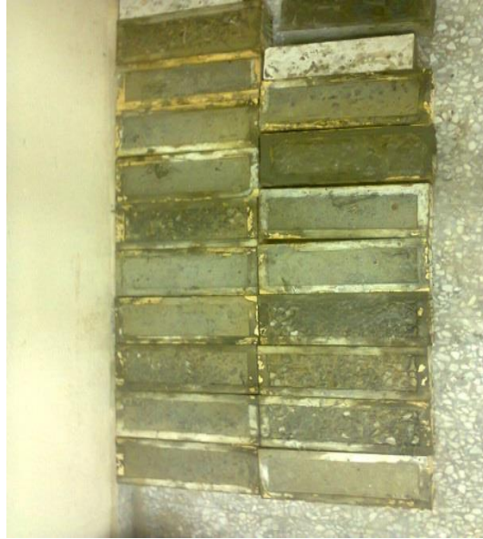
Figure 3.16 : beam mold for shrinkage test 75x75x250mm
